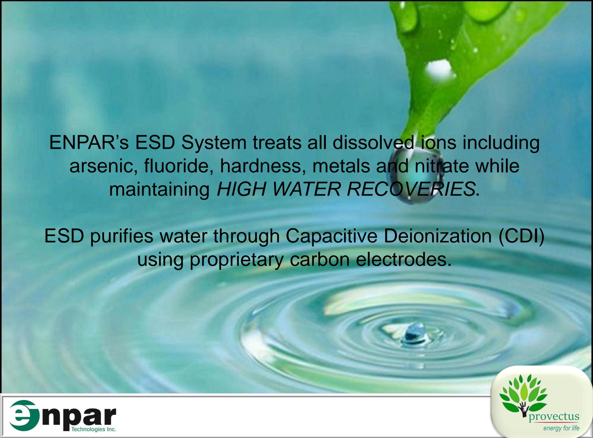
ENPAR's ESD System treats all dissolved ions including arsenic, fluoride, hardness, metals and nitrate while maintaining *HIGH WATER RECOVERIES*.
